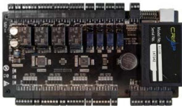
CRISP's CON-X is an enterprise-grade series of Access Control panels supporting advanced web-socket based real-time auto-push communication protocol. The panel support features such as anti-passback, first-card opening, multi-card opening, duress password entry, embedded card verification & auxiliary input/output linkages.
